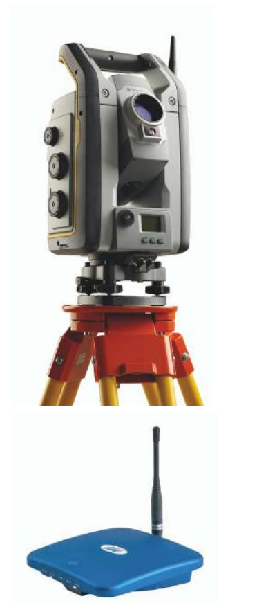
Figure 3: Key components - (Top) Trimble S7 Total Station and (Bottom) the Trimble Settop M1 controller.
