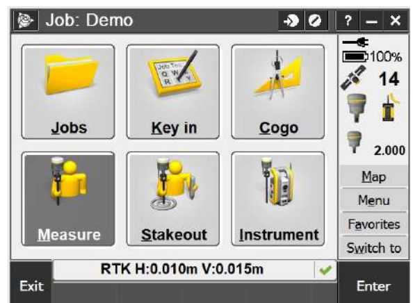
Figure 3: Trimble Access software enables surveyors to combine GNSS and total station data for resection, stakeout and in-field computations.
