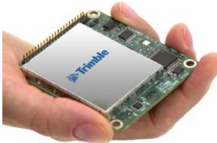
Figure 4: Integrated GNSS/INS for Precision Survey and Mapping.
