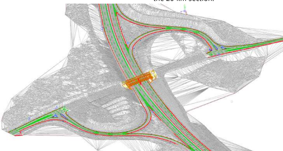
Figure 3: A section of the A93 highway combining vectorized break lines from the MX9 data and a DTM..
