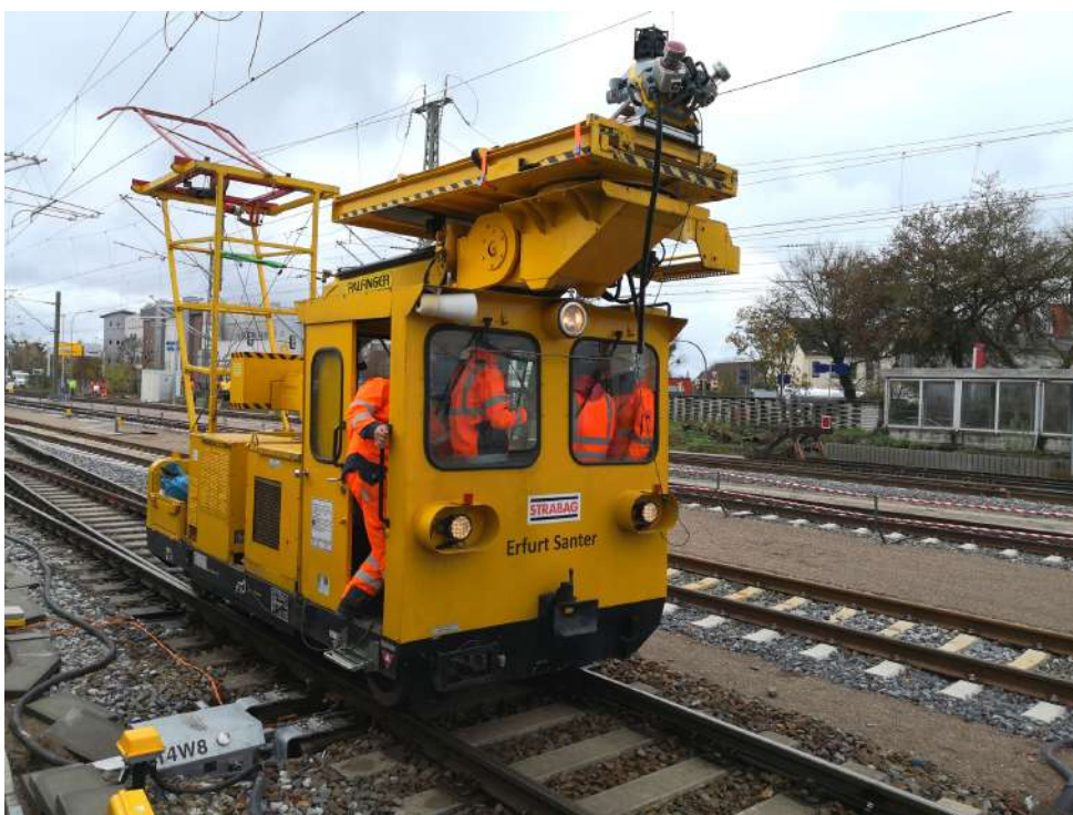
Figure 7: The MX9 mobile mapping technology is an asset on railway projects because it can scan overhead power lines, which are complicated to survey with a tachymeter.
