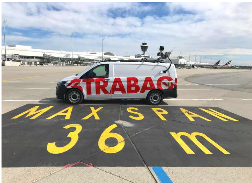
Figure 4: The MX9 3D mapping system sits ready to capture data at the Munich Airport.
