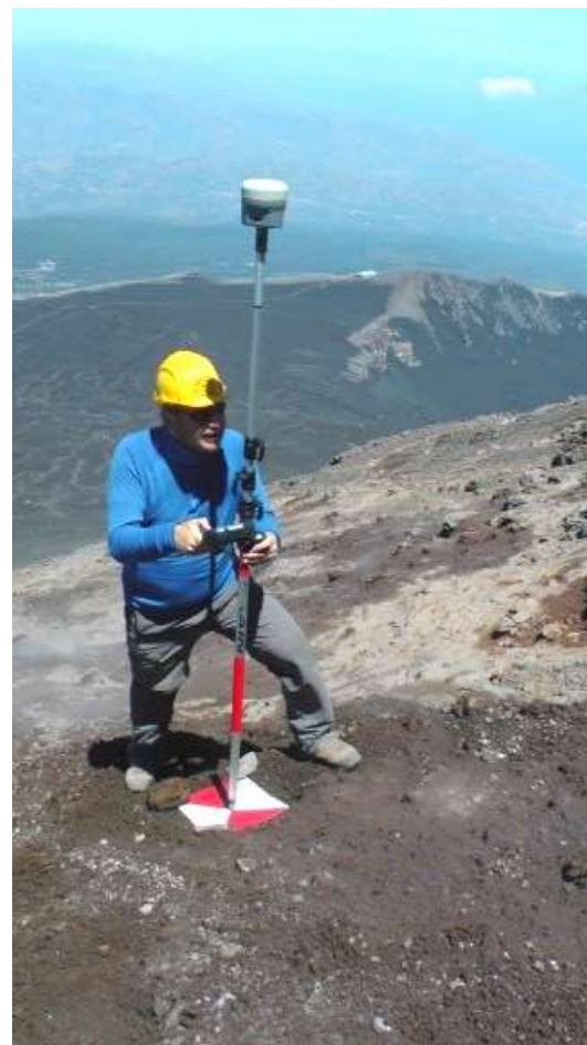
Figure 1: Juraj Papčo measures a position for topographic mapping high on Mount Etna. Measured points were compared with models created from aerial imagery.
