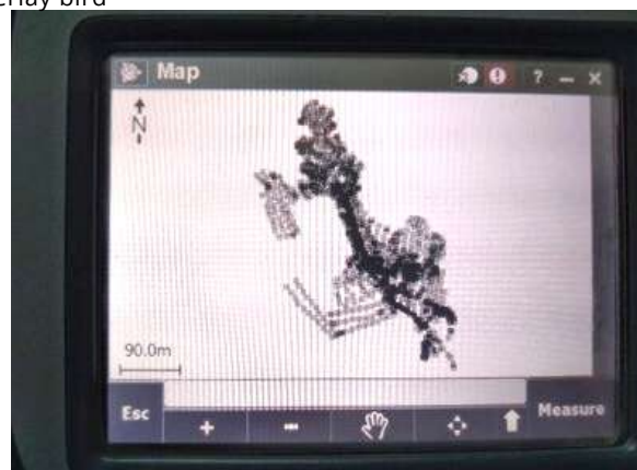
Figure 2: The TSC3 displayed all the points captured with GNSS. The data were later transferred to CAD software for mapping and design.
