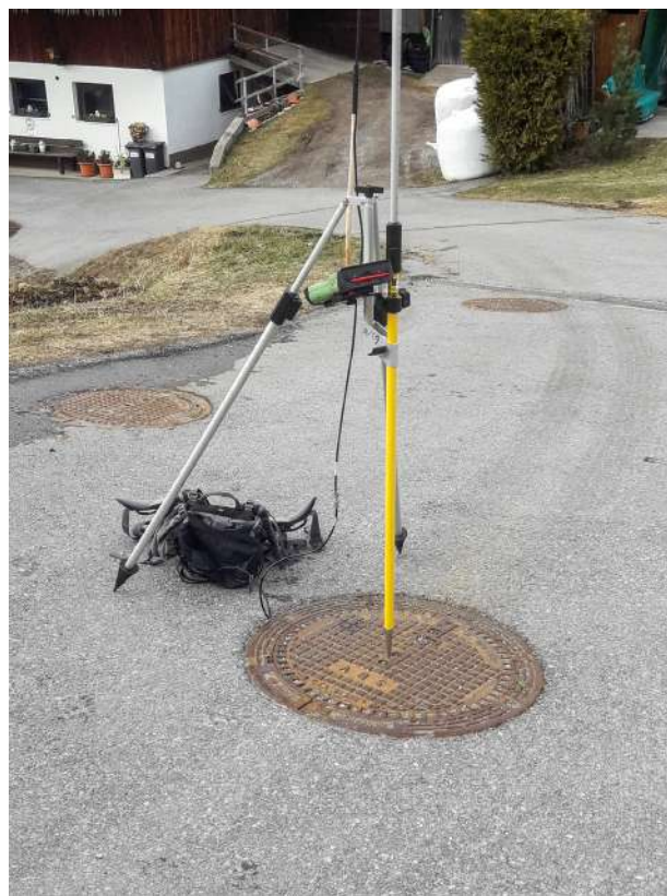
Figure 2: One of 50 ground control points AVT set out to establish control for the flight.
