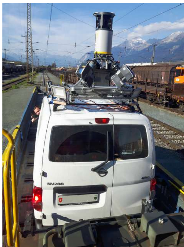
Figure 3: The Trimble MX7 mobile imaging system was mounted on the roof of a small van and pulled by a special locomotive of the ÖBB. The Trimble MX7 captured ancillary features not visible from the plane.
