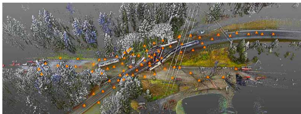
Figure 6: Gunderson integrated scanning data and UAV photos into Trimble’s RealWorks software to create a 3D point cloud of the incident scene. In this view, orange markers indicate the location of each of the 82 set ups taken with the Trimble TX5.
