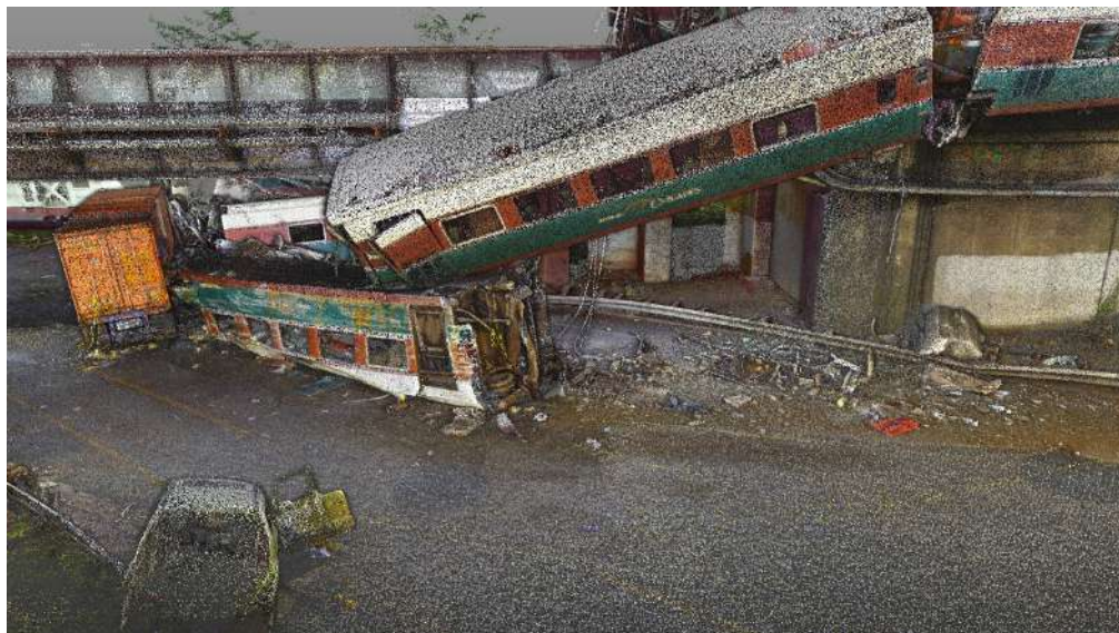
Figure 4: Wreckage from the Dupont train derailment captured by a Trimble TX5 laser scanner. In total, four teams collected 82 scans and more than one billion data points in five hours.
