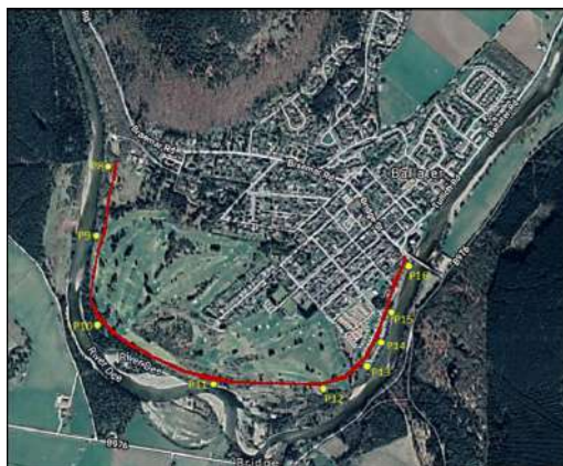
Figure 18: Extent of computational domain around the town of Ballater in test CASE 4. Proposed flood defence barrier (red) and probe sampling points are also highlighted.
