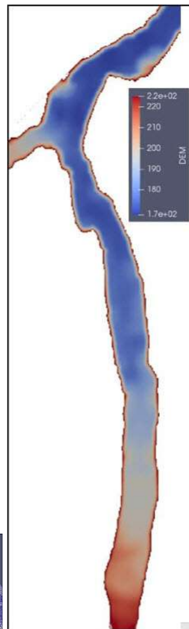
Figure 5: Valley DEM generated using OpenFOAM utility Test-WallDist.
