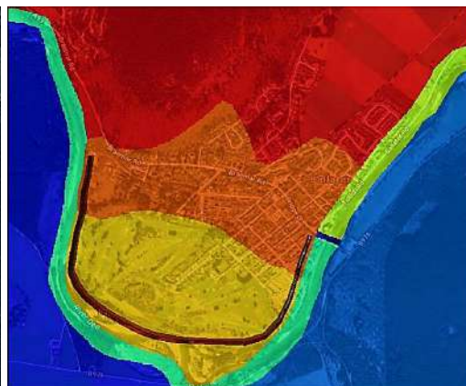
Figure 19: Roughness zones for different Manning-Strickler coefficients in test CASE 4.
