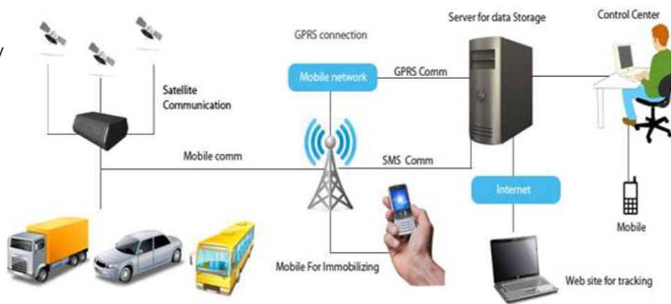
Figure 5. Various technologies and components of LBS tracking system
