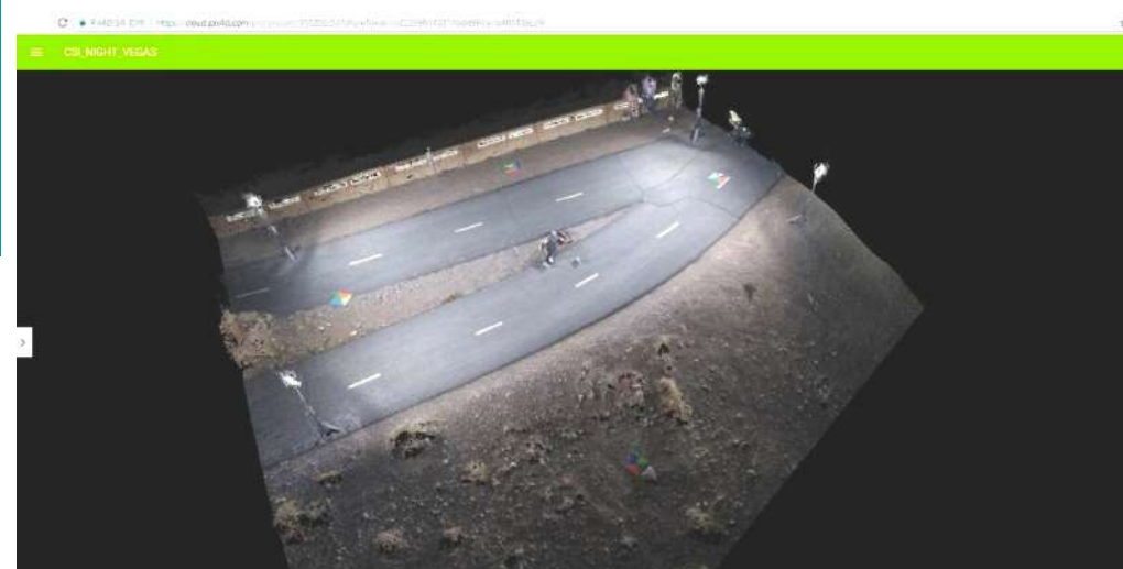
Figure 3: Processing images with Pix4D drone mapping software.
