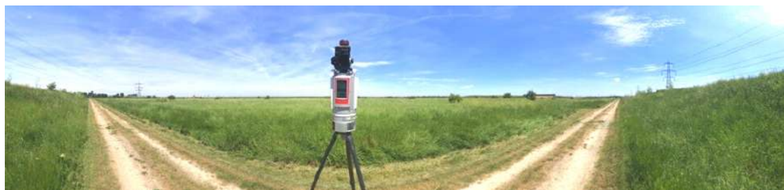
Figure 6: Rural featureless scene, registered automatically without targets, 40m intervals.
