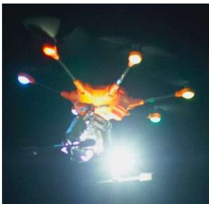
Figure 4: With specially-designed lights, drones can be used at night to capture images.
