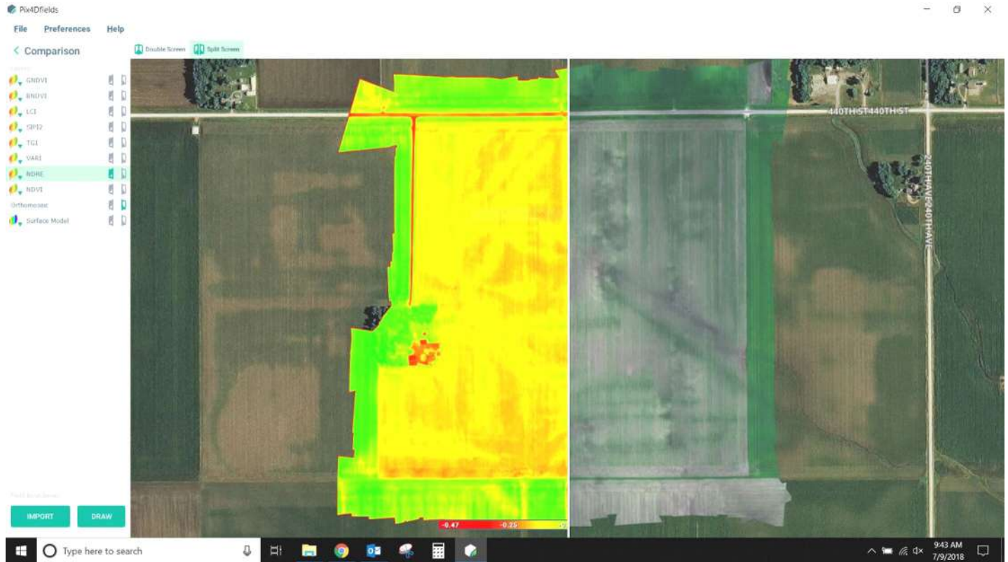
Figure 3. NDRE index vs orthomosaic using the split-screen comparison tool in Pix4Dfields.
