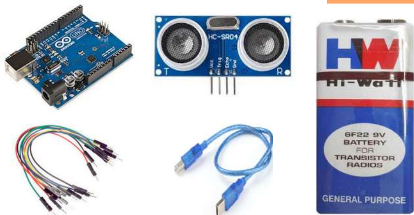
Figure 3: Arduino Uno, Ultrasonic Sensor (HC-SR04), Jumper Wires, USB Cable, 5V Battery (Top to Bottom - Left to Right).
