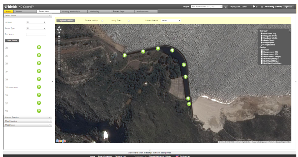
Figure 6. Trimble 4D Control's customizable view that allows users to import pictures of their specific structure for easier visualization.
