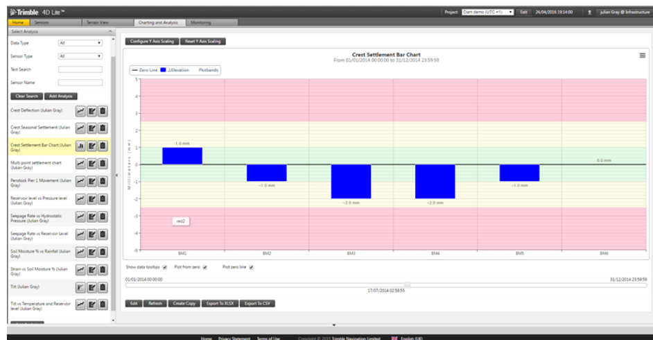
Figure 2. Visualization of the displacement and/or settling of the dam. In this case, for the crest of the dam..
