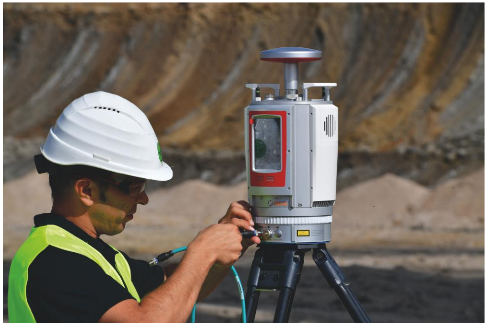
Figure 1. RIEGL VZ-2000i 3D Terrestrial Laser Scanner
