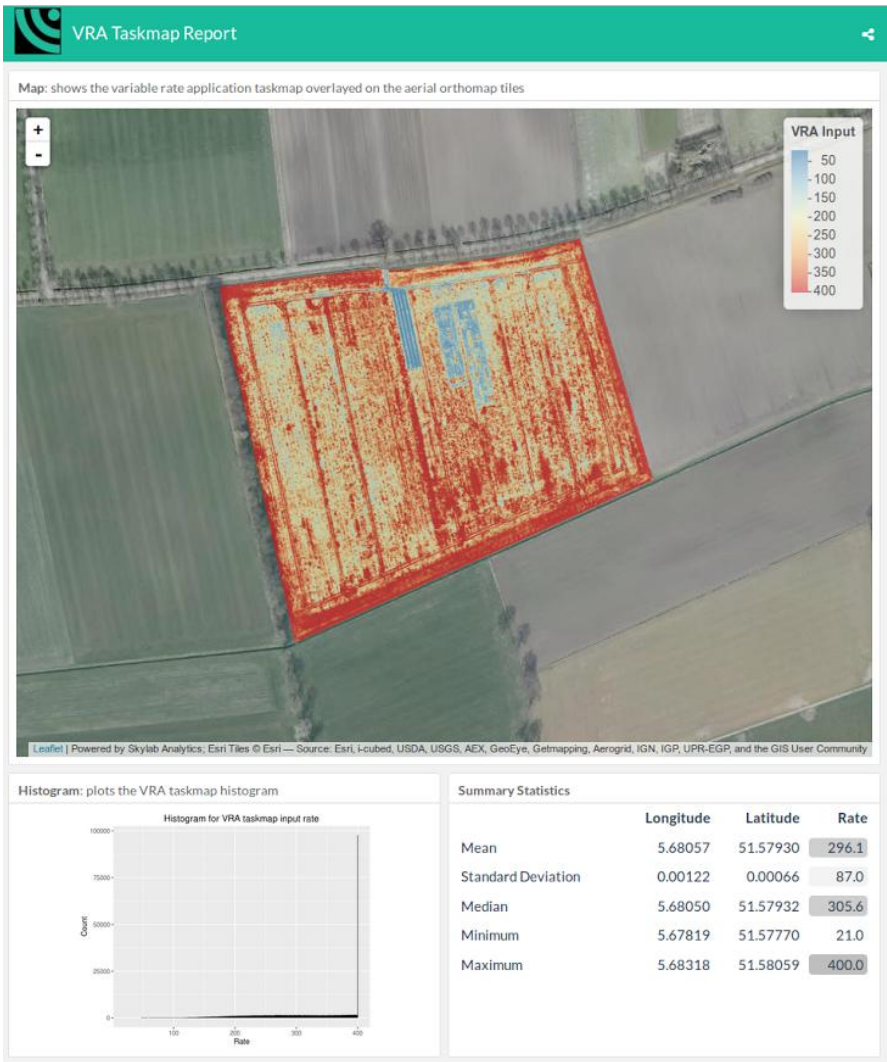
Figure 1. Automatically generated VRA taskmap enabling the input where and on the quantity needed
