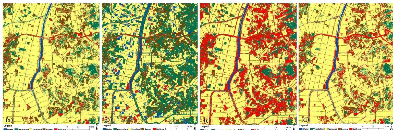
Figure 3. Land cover classification of the test site using ratio and indices bands composite: (a) MahD; (b) MinD; (c) ML; and (d) SVM
