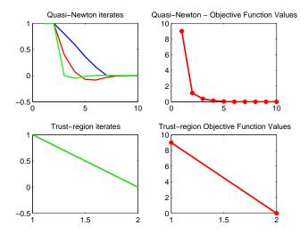
which indicates that the LargeScale option of fminunc applied to the problem in func1.m converges after a single iterative step. (Compare also the tables that will be displayed when running TestFminunc.m).
