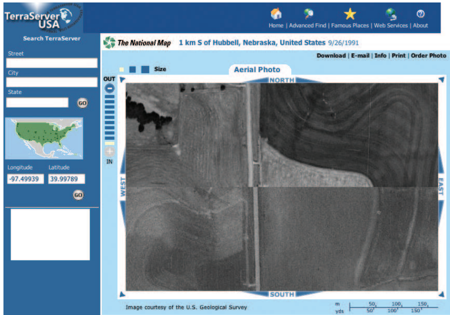
Figure 4.2: An example of misregistration
